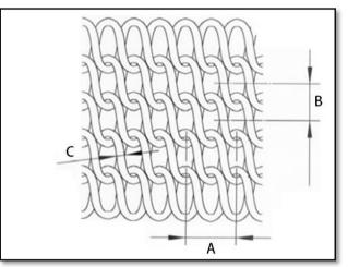
**NOTE:** When measuring pitch, it is best practice to measure over 10 double coil pitches (20 individual coils) and then divide by 10 to obtain the average double pitch.
